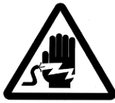
Caution: Shock Hazard!
